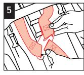
Fit loops on harness ends onto the splitter plate.
